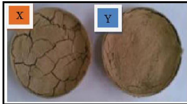
Fig. 7 Aridness cracking (X) unreinforced sample (Y) reinforced sample
